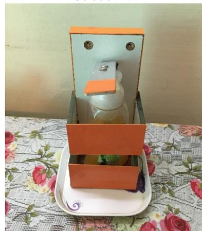
**Liquid handwash dispenser fitted with forearm/elbow operable lever**
