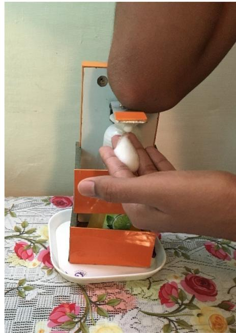
4. It can easily be operated by forearm/ elbow. This holder can accommodate most commercially available handwash dispenser bottles.
