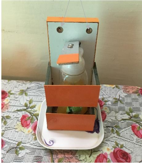
3. The aluminium strip is affixed with a hinge into a suitable holder, made of scrap plywood and laminate. It may be wall-mounted. Provision of wall fixing is made.
