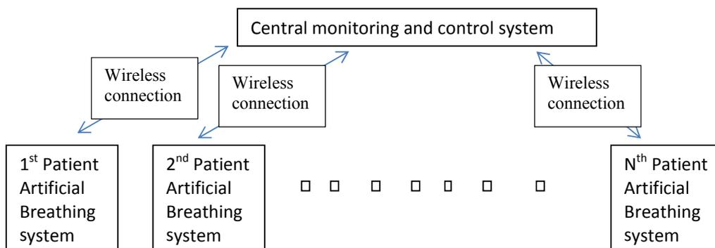
Fig. 6 Wireless monitoring and control of multiple Patient Artificial Breathing systems
