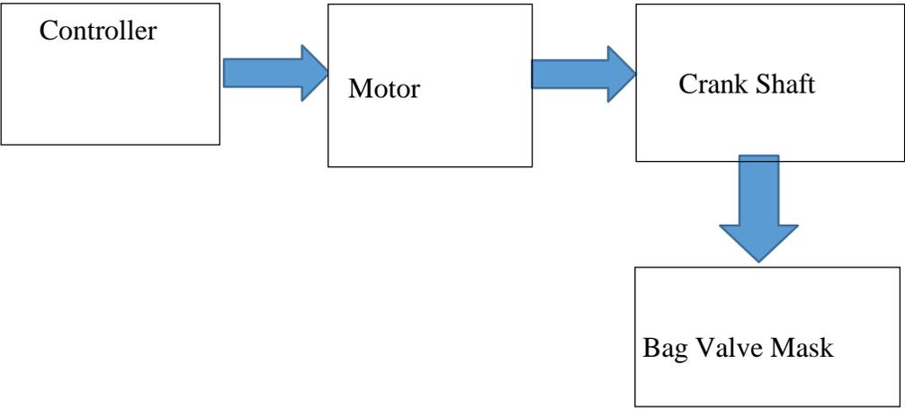
Fig1: Schematic flow diagram of an open-loop Automated artificial breathing system
