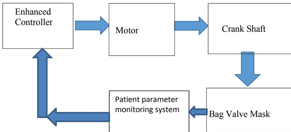
Fig5: Schematic flow diagram of a closed-loop Automated artificial breathing system
